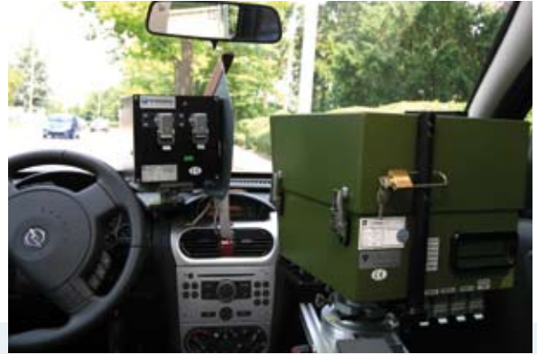
PoliScan speed installed in place of the front passenger seat ...
