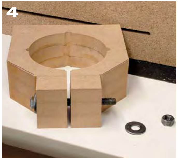
4 Cut the collar to shape using your table saw or band saw. Then stand the collar on edge and drill a \frac{3}{8} "-diameter hole for the bolt.
