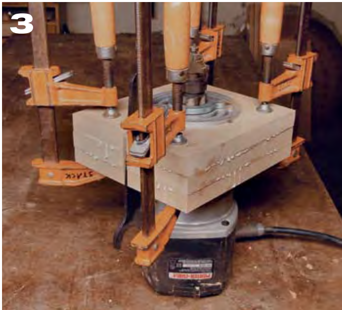
3 To hold the three collar pieces in alignment, I used my router as a form. Use enough glue to hold the parts together but keep the glue away from the inner edges of the circle cutout if you can. If a little glue does stick to your router's body, simply pop off the dried glue with a chisel.
