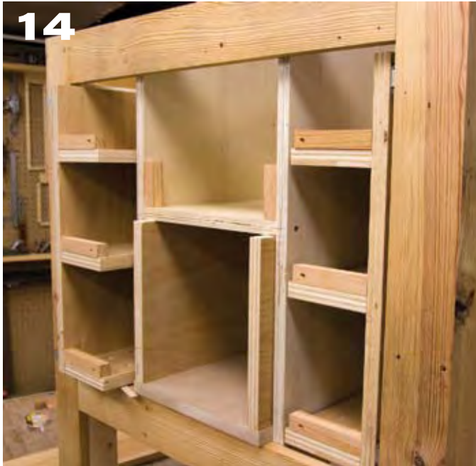
14 Glue cleats to the pullout shelves, to the sides of the top space and to the sides of the drawer (I haven't glued these in place yet).
