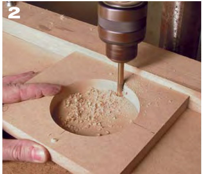
2 If your router has those little tabs on its body like mine does, you'll need to cut out for those so the collar will slip on the router's body smoothly.
