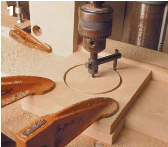
1 Cut out three collars for the router collar assembly. In each collar, cut a hole larger (add \frac{1}{16} " to the diameter) than the diameter of your router's body.
