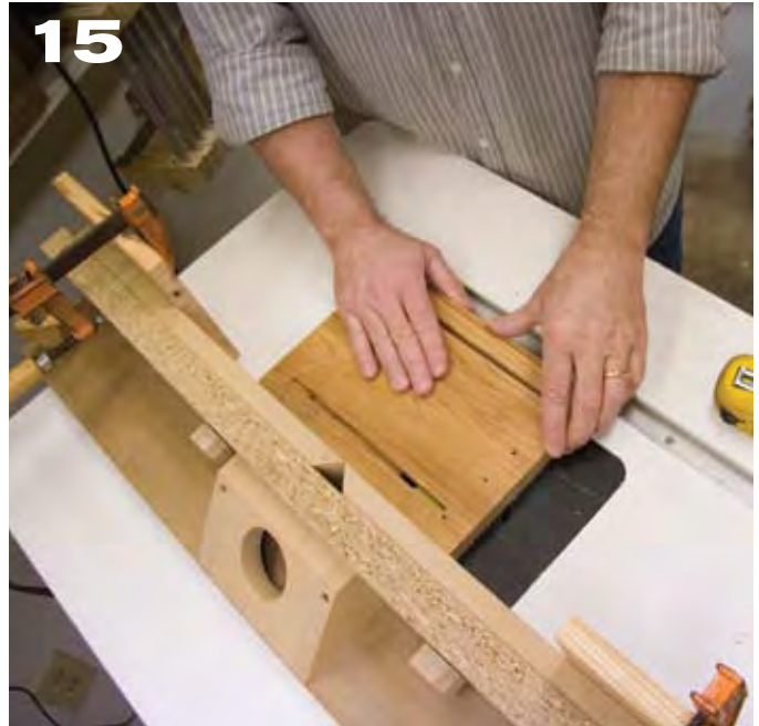
15 Cut out the drawer front, pullout fronts and the vent panel. Fit them to the front of the router table, leaving about \frac{3}{32} " space between all these parts. Then cut the vents in the vent panel. Here, I am using my old router table to plunge-cut the vent slots.
