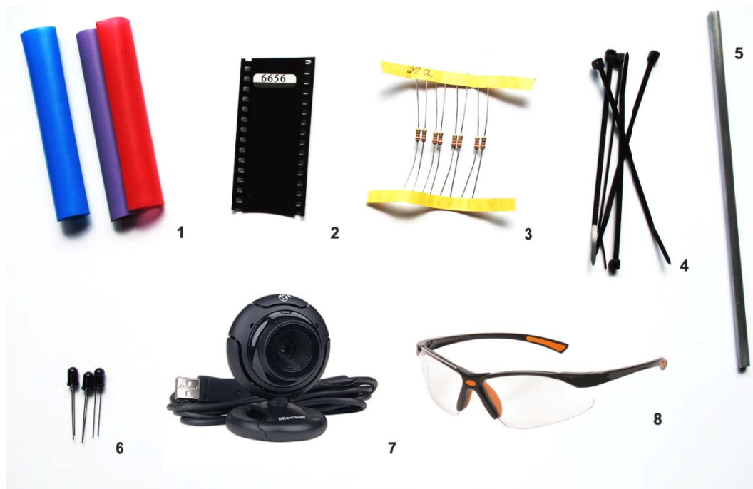
Figure 1.1: Elements of eye gaze tracking glasses: 1) heat shrinkable tubin, 2) negative film, 3) carbon resistor, 4) mounting strips, 5) aluminum wire, 6) IR LEDs, 7) Webcam LifeCam VX-1000, 8) safety glasses
