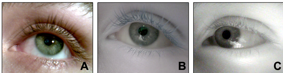
Figure 2.2: The eye image obtained from a camera: A) without modification, B) without the filter of visible light, C) with IR filter
