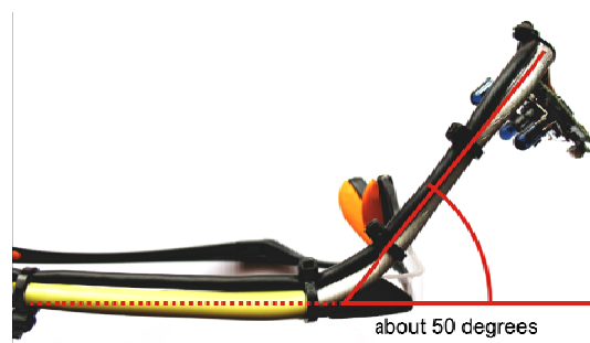
Figure 3.3: Bending angle of aluminum wire
